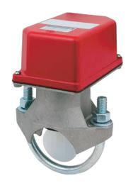
They are used in sprinkler system to transmit electrical information due to the flow, when a sprinkler head gets activated. Delay units are available to prevent false alarms.
