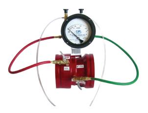
It is used for periodical control of the pump systems whether the desired flow rate is achieved. The flow meter is usually mounted between check valve and OS&Y valve in pump discharge lines. The diameter of the flowmeter is determined by the pump flow.
